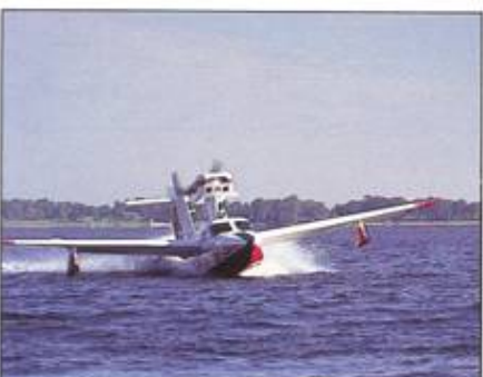
No special ramps are required for beaching if the shoreline is fairly smooth. Lower the gear and forge on.
