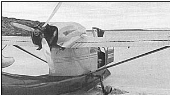
The right gear has rolled into the hole dug for it, waiting for high tide. If the tide were not present, and thus not a factor, more digging would be required.
