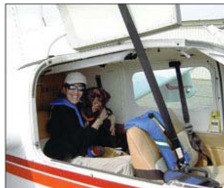
Clifford Maine's wife Betsy and their flying buddy. The cargo hatch is a welcome feature. Earlier Lakes didn't have it, although it's available as a mod.
