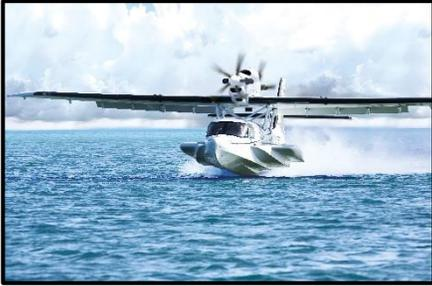
Note the lack of wing floats, as the *sponsons* protruding from each side of the hull preclude the need for them.
