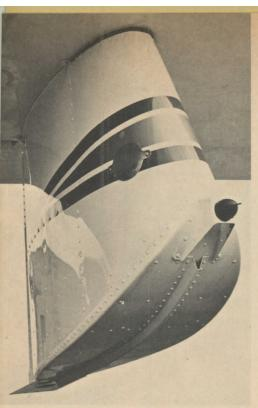
Flat-bottomed floats act as skis, so wing won't dig in on turns. The round stainless mirror allows the pilot to check nose gear position.
