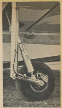
Taxiing on the water, the lowered landing gear makes excellent speed brake (left). Main gear, above, is of stainless steel, retracts inward.
